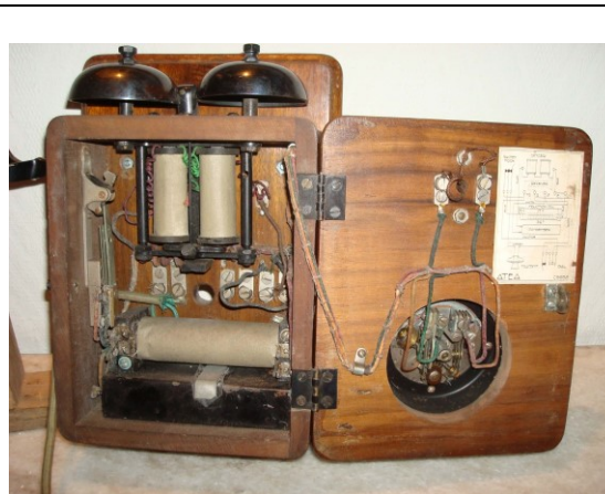
Figure 2: Remarkable ATEA telephone- inside view
