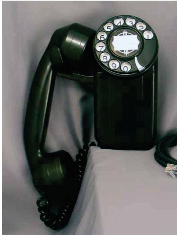
Fig. 15 - Automatic Electric Model 43 Spacemaker with zinc alloy body
