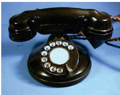
Fig 3: The ATM Strowgerphone ATM made basically the same phone as AE, The major difference was the BPO type 164 handset.
