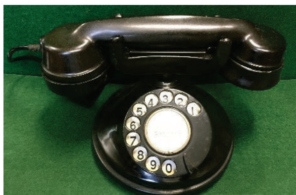
Fig 6: Automatica Electrica Portuguesa (AEP) version Automatica Electrica Portuguesa was a British/Portuguese company owned by ATE. It used the standard GPO handset. John Mulrane (IRL) has such a Portuguese monophone. It was built in the 1950s.
